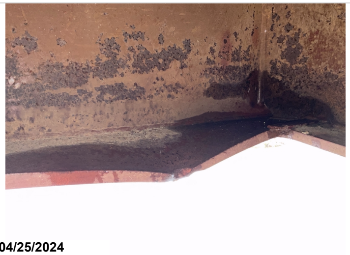
Left Railcar, Girder 1, 1' back of Floor Beam 2: out-of-plane bending.
