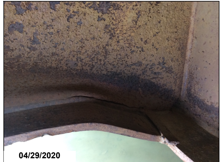
Left Railcar, left Floor Beam - 8" horizontal crack at bottom flange.
